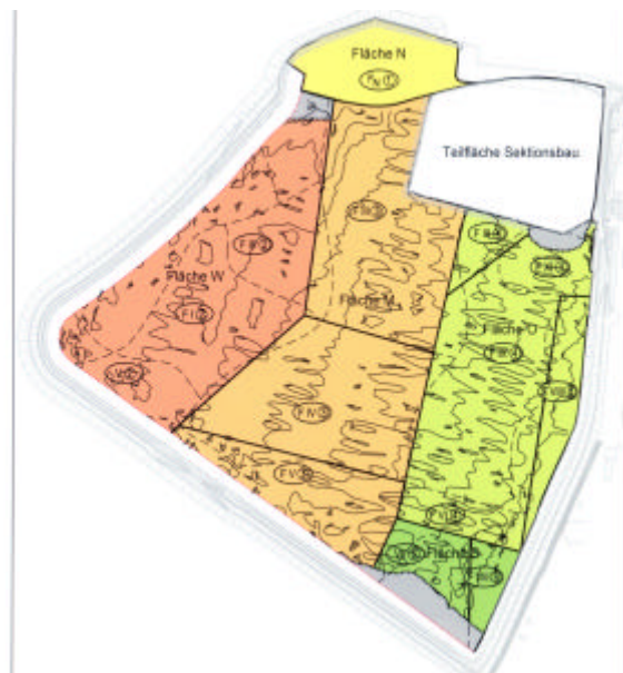
Figure 10. Division of the area for filling of the first sand layers
